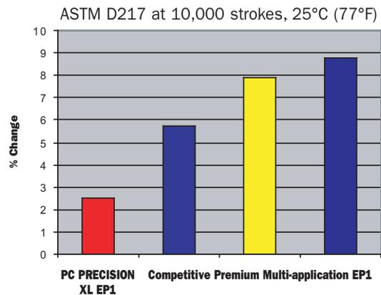
\*The significance of the tests is to demonstrate the stability of the grease under normal and moderate shear conditions. The lower the number in the graph, the better is the grease performance, and the longer its service life.
