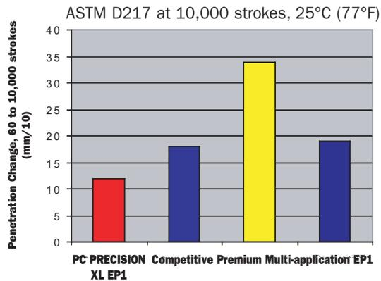
**PC PRECISION XL EP1 with the lowest break-down under moderate shear conditions provides stability and longer service life for customers**
