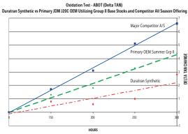
\*Note: Results are after 300 hr ABOT Oxidation Test which is more severe than JD requirement Allison C-4 ( GM 6137M) Oxidation Test.
