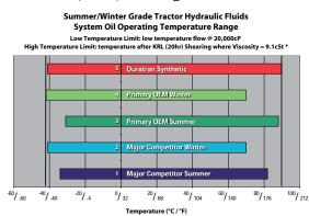
Minimum viscosity is  $9.1cSt @ 100^{\circ}C$ . The after-shear temperature at 9.1cSt shows the stability of the fluid (higher is better).
